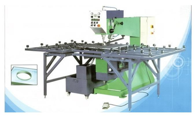
Throat depth: 1200mm (47 1/4") Hole diameter: 4-160mm (3/16" - 6 1/4") Glass Thickness: 3-30mm ( 1/8" - 1 3/16") Support table: 600mm x 500mm ( 24" x 20") Table height: 900mm ( 36") Weight: 850kg ( 1,870 LBS ) Machine size1950mm x 850mm x 1800mm ( 77" x 33" x 71" ) Support table: 2000mm x 1380mm x 850mm ( 78" x 55" x 33" ) Power: 220 Volt, 3 phase, 60 Hz Motors: 1.1 Kw x 2 Air supply: 0.6 Mpa
